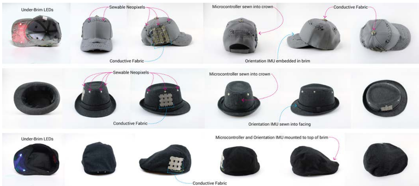
Figure 9. Hat prototypes capable of sensing touch and head gestures. The baseball cap (top) has ambient displays under the brim and across the crown; the fedora (middle) has an ambient display across the crown; and the flat cap (bottom) has an ambient display under the brim. In all three prototypes, the battery is tucked into the facing on the inside of the crown.
