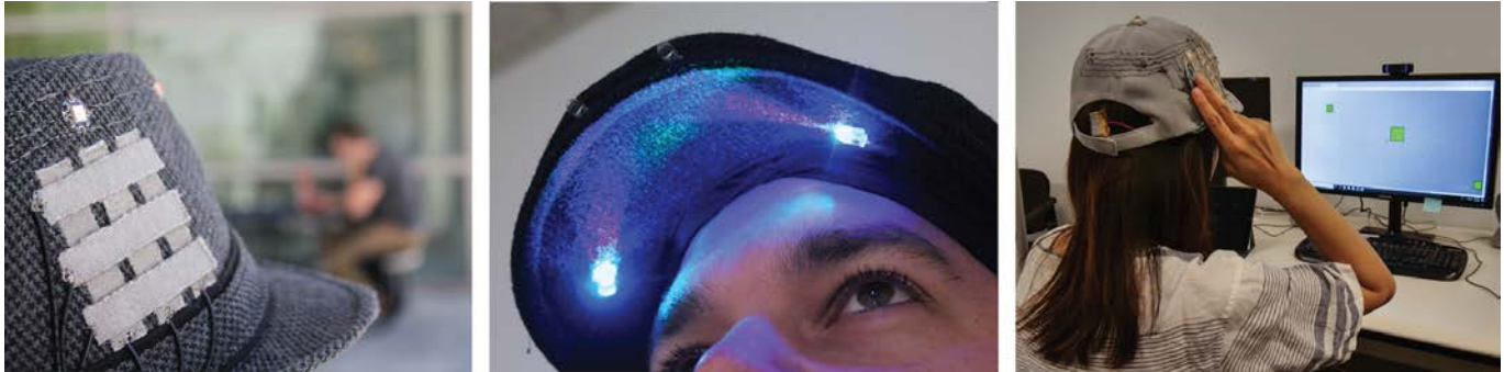
Figure 1. Left: touch sensitive region and public crown display of the fedora prototype. Middle: personal under-brim display of the flap cap prototype. Right: user evaluation of our baseball cap prototype.
